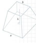
For this particular frustum, the function  $V(x) = 0.5x^3 - 3x^2 + 6x$  can be used to calculate the volume when a = x, b = x - 6, and  $b = \frac{1}{2}x$ .
